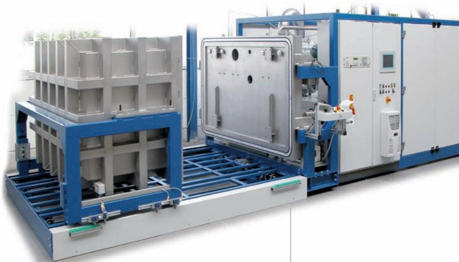
Helium leak testing equipment for
