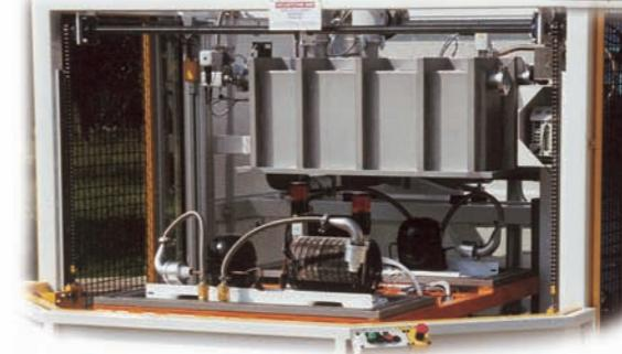
Helium leak testing equipment
